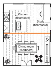
If there was damage to the flooring at the spot marked 'X' in the dining room, we would only repair or replace the flooring within this functional area up to the orange line. In this scenario, we may need to introduce a floor trim along the orange line.
