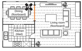
If there was damage to the flooring at the spot marked 'X' in the dining room, we would only repair or replace the flooring within this functional area up to the orange line. In this scenario, we may need to introduce a floor trim between the dining room and living room along the orange line.
