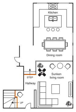
If there was damage to the flooring at the spot marked 'X' in the sunken living room, we would only repair or replace the flooring within this functional area up to the orange line. In this scenario, we may need to introduce floor trims at the base of the steps along the orange lines.
