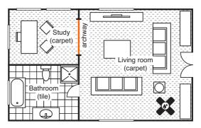
If there was damage to the flooring at the spot marked 'X' in the living room, we would only repair or replace the flooring within this functional area. In this scenario, we may need to introduce a floor trim between the study and living room as per the orange line, since the damage is contained within the living room alone.
